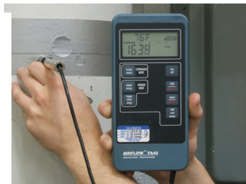
Right: Anemometer measures air flow.
